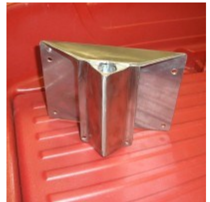
The bracket fastens to the back of the wagon and allows parents to transport patients without worrying about the IV pole.
